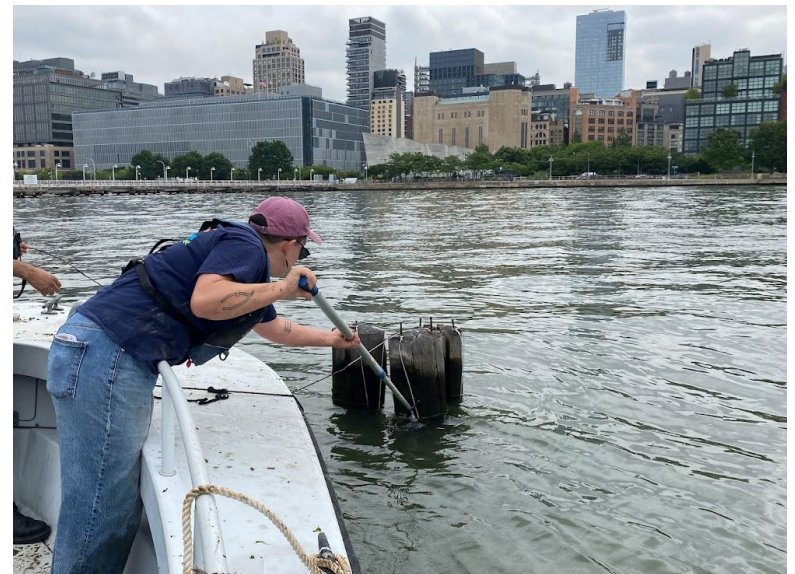
Fig. 10 | Retrieval of wraps off a pile with a boat hook in June 2023.
