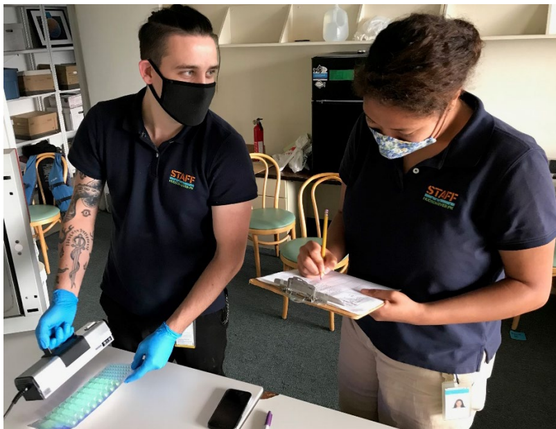
Figure 56: The Park's River Project staff reads pathogen results from incubated water samples dispersed in an IDEXX Quanti-Tray using ultraviolet light.
